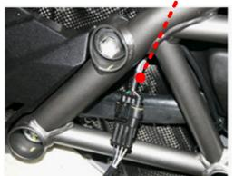
QuickShift connection Is on right hand side of frame using Horizontal O2 plug
